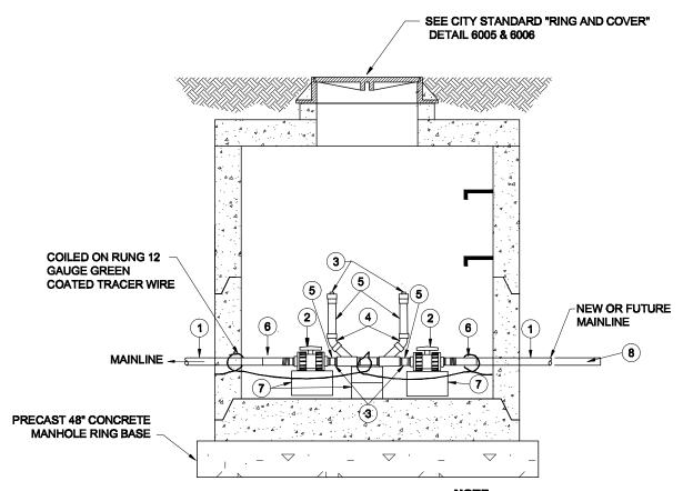
INSTALL PLUG IN THREADED TEE OR FUTURE **EXTENSION FOR TERMINAL CLEANOUT**
