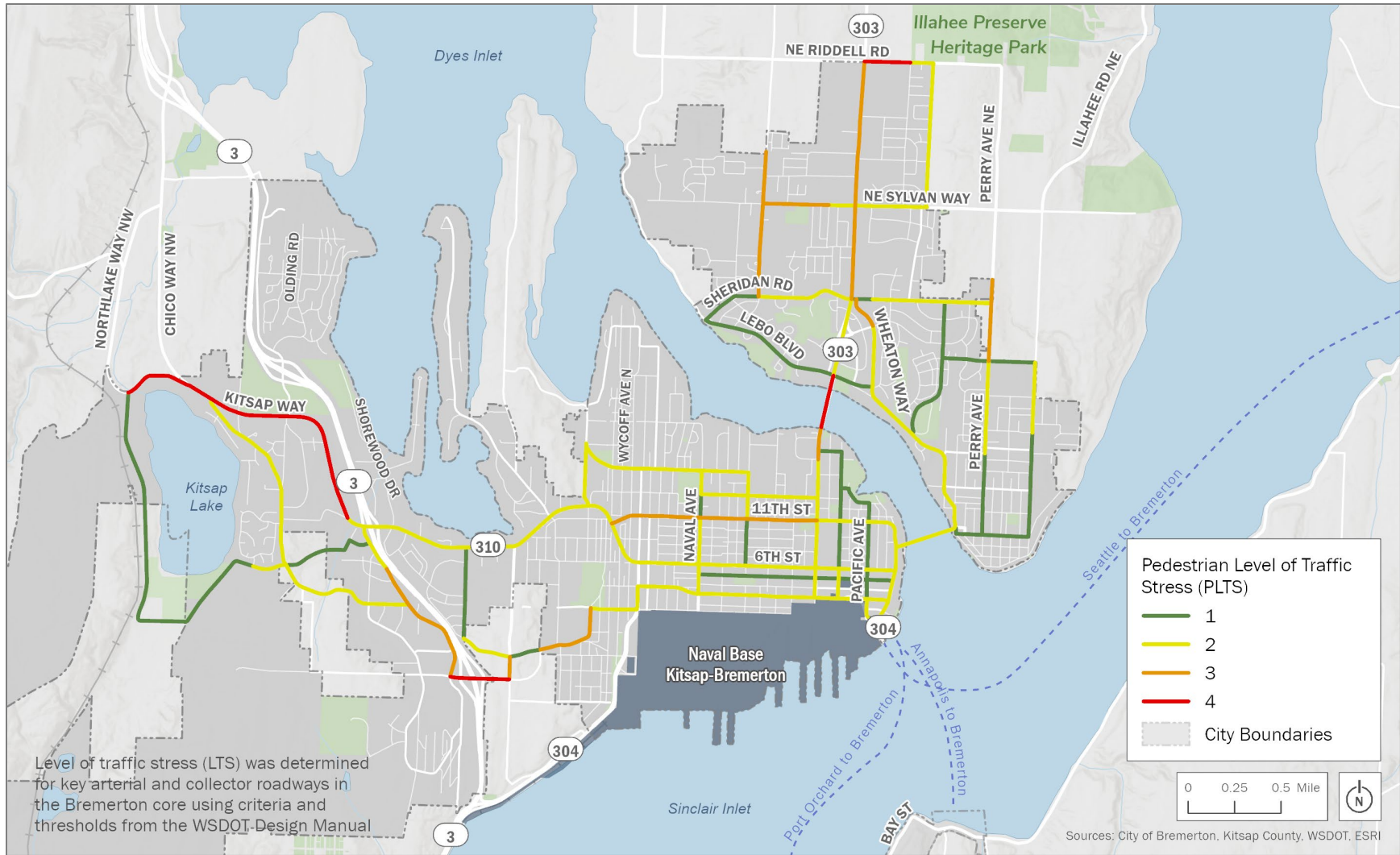
Figure 17. Existing Pedestrian Level of Traffic Stress (PLTS) on Arterial and Collector Roadways
