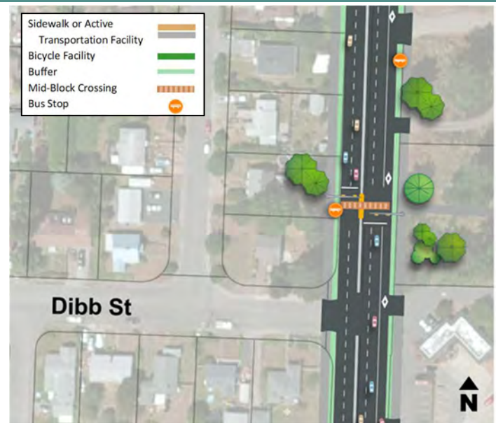
Note: Conceptual drawing only. Channelization and sidewalk improvements are not included in this phase.
